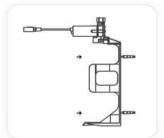
5. Assemble the tube from the pump to the soap dispenser.
